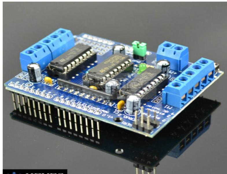
L293D is a monolithic integrated, high voltage, high current, 4-channel driver. Basically this means using this chip you can drive DC motors with power supplier up to 36 Volts, and the chip can supply a maximum current of 600mA per channel. L293D chip is also known as a type of H-Bridge. The H-Bridge is typically an electrical circuit that enables a voltage to be applied across a load in either direction to an output, e.g. motor.
